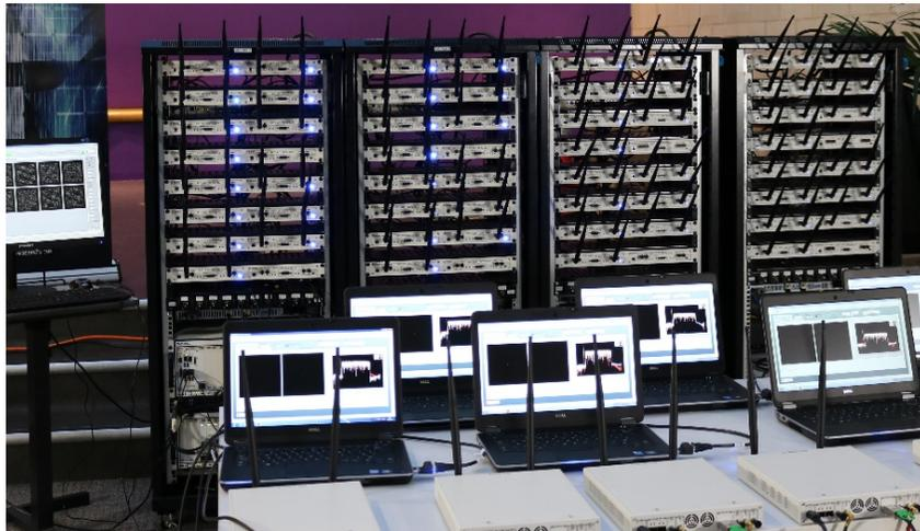
Validating massive multiple input, multiple output (MIMO) as a technology that can bring huge capacity and energy efficiency gains to future 5G networks, which must accommodate increased data rates and the rapid proliferation of smart connected devices, without consuming any more of the radio spectrum.
