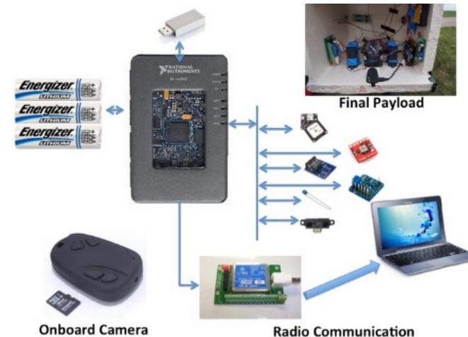
Using **myRIO** to control all on-board sensors and experimental equipment in a high altitude balloon, from the launch to the landing with real time monitoring and post processing.
