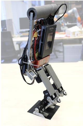
Implementing learning and control algorithms for squat movement and autonomous balance management on a walking Bipedal Humanoid Robot
