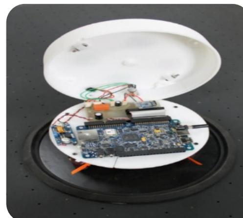
Developing small robotic devices based on the NI myRIO and using LabVIEW to write the code, including the robot software and the ground station platform, all with space-like computers, software, sensors, and actuators.
