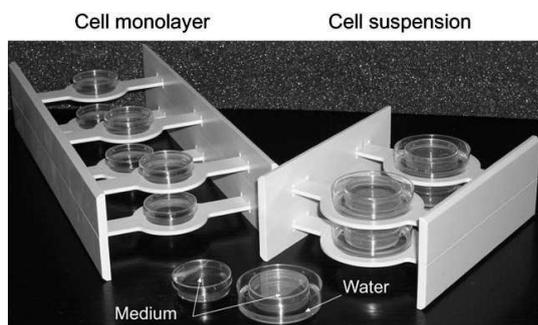
Fig. 2. Petri dish holders for cell monolayer and cell suspension [7]
