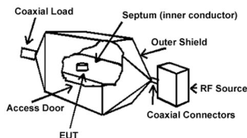
Fig. 1. Standard construction of the TEM-cell
