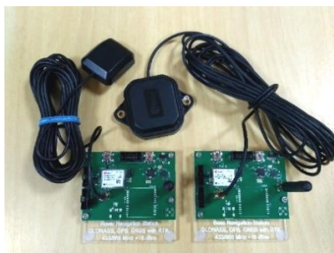
Fig. 1. Test set of the navigation system
